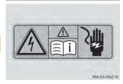
The components of the drive system are indicated by yellow warning labels to make you aware of high voltage.
