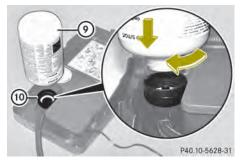
► Screw tire sealant container ⑨ onto flange ⑩.
