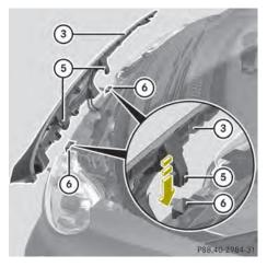
▶ Insert hooks (5) on the back of service flap (3) into openings (6).
