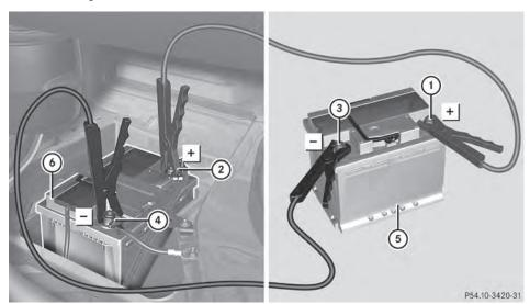
Position (5) represents the charged battery of another vehicle or an equivalent starter pack.
