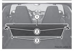
If you wish to use cargo compartment cover blind ① as normal, assemble it in top mountings ②. If you do not need the cargo compartment cover blind, insert in bottom mountings ③.
