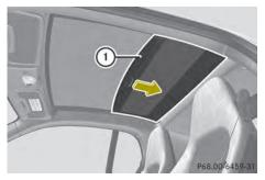
▶ Opening or closing: Move sun screen ① forward or backward using the handle.
