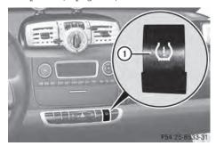
▶ Press Restarting TPMS button (1). The combination low tire pressure/TPMS malfunction telltale in the instrument cluster (⊳ page 21) flashes for approximately 5 seconds and then goes out.
