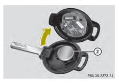
▶ Remove transmitter battery ② from the board.
