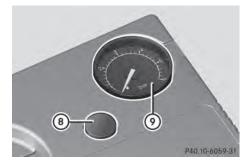
► Check the tire inflation pressure using pressure gauge ⑨.
