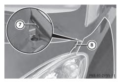
▶ Insert left and right links (8) of service flap (3) under links (7) on the fender.
