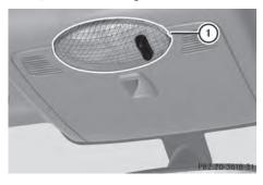
▶ **Removing:** Use a flat object to pry the lamp lens (1) off from the passenger side.
