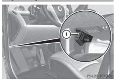
Your vehicle is equipped with a high-voltage disconnect device ① to disable the vehicle's high-voltage system.
