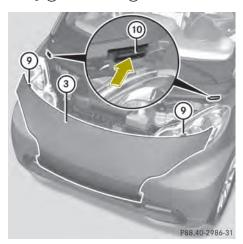
▶ Insert both tabs (9) on the back of service flap (3) completely into openings (10).
