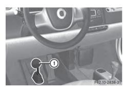
If a brake circuit has failed (▷ page 160), you must depress brake pedal (1) further down to achieve the same effect and the braking distance is increased.
